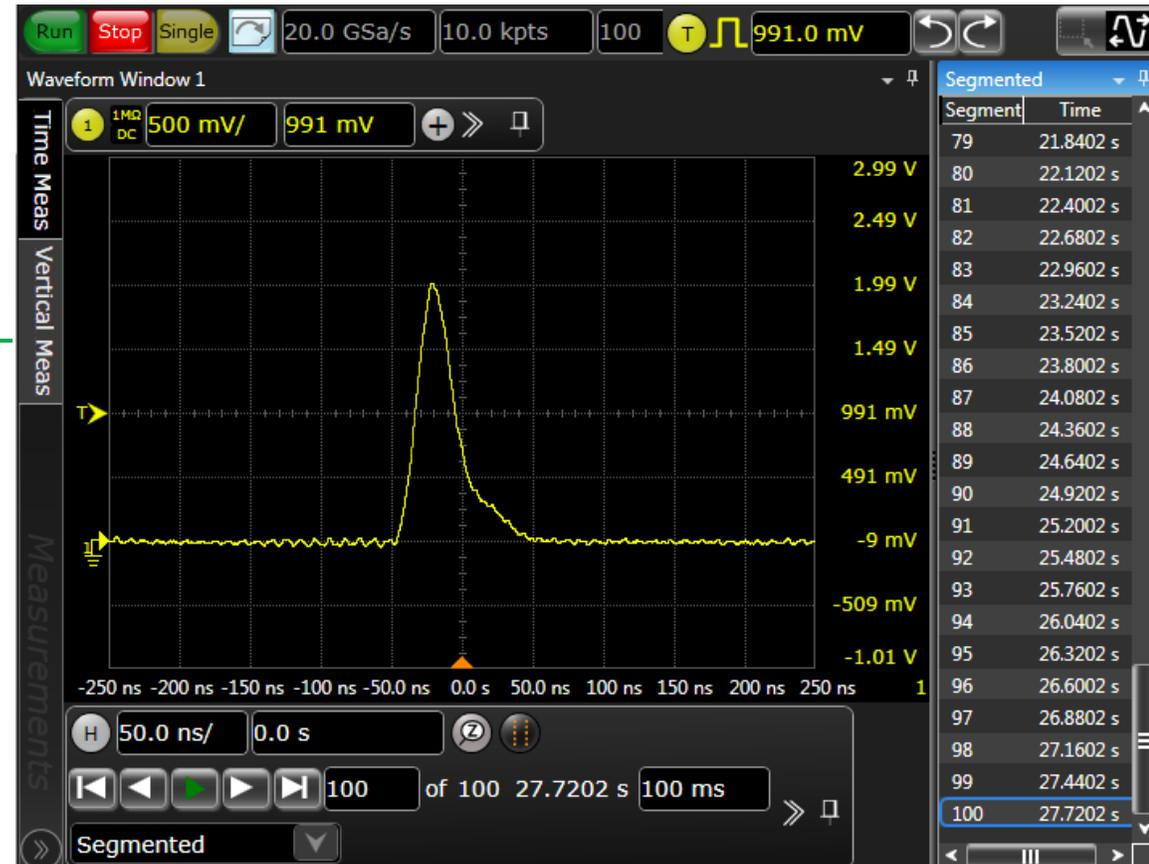
Equivalent Memory = Time-span x Sample Rate
