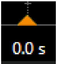
0 seconds (trigger point) is shown with an orange triangle, and can be adjusted left and right.
